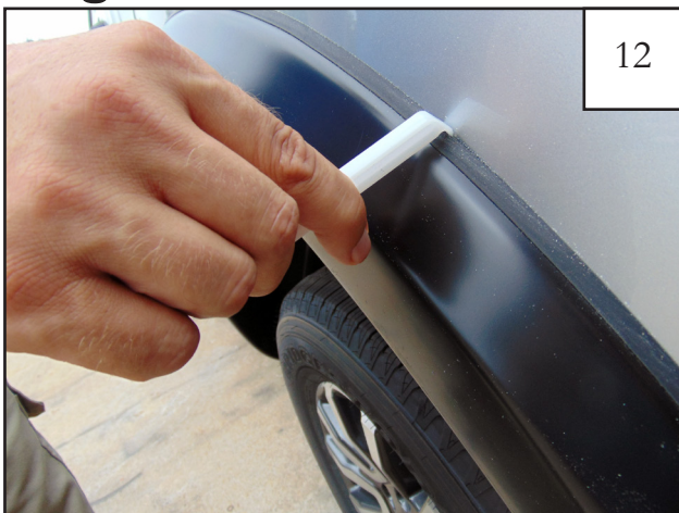
12 Using supplied Edge Trim Tool (ET1-0002), seat edge trim against vehicle by hooking curved end under edge trim at one end of flare. Next, slide around outer edge of flare to the other end.
