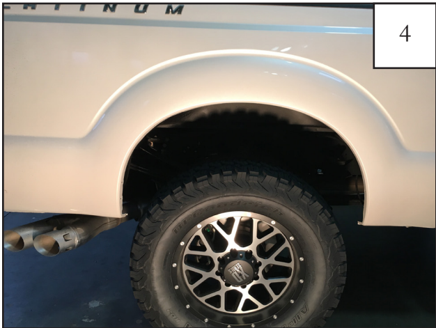
Hold flare to vehicle and ensure that the four holes in flares line up with four factory holes in the fender.
