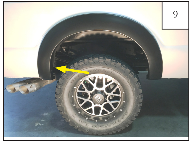
9 Install a 5/16" Phillips Truss Screw (SW1-0050) into the "S" clip over the rear most hole.
