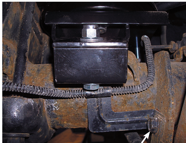
It may be necessary to adjust the brake line bracket slightly to gain clearance to insert and tighten the rear left (driver's side) hardware as shown.
