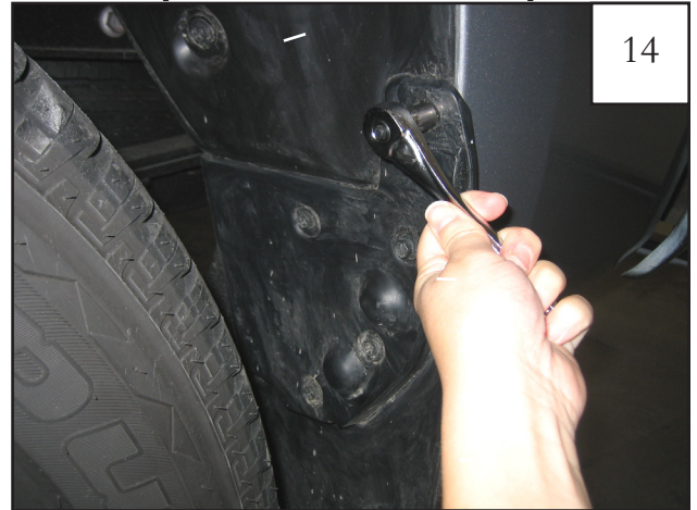
Remove top screw from mud flap as shown.
