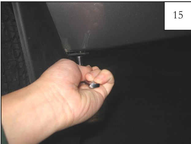
Remove screw from underside of factory mud guard.
