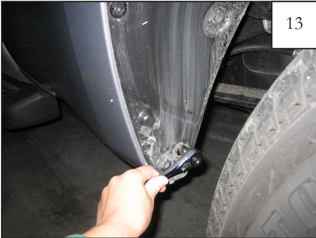
Using a socket wrench with a 10mm socket, remove lower screw from front of rear wheel well as shown.
